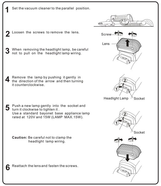
**Caution:** Be sure to turn the ON/OFF switch to the "OFF" position and disconnect the power cord from the wall outlet before replacing any of the parts below.
